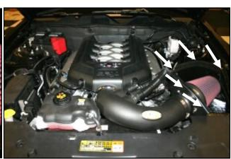
13. Reconnect the Mass Air Flow sensor, which is now 14. Install the Weather Strip (#7) onto the CAB with the located in the lower back side of the intake. Slide the contoured edge going away from the filter. Start at the front of the vehicle and work your way back. Replace the
