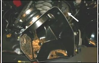
7. Transfer the factory air box mounting grommets. A) 8. Install the hump hose (#4) onto the filter adapter using two #72 hose clamps (#11) as shown. Leave the two hose clamps loose for now. Transfer the resonator stand
