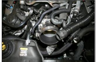
**10.** Install the Silicone Reducer (#5) and Hose clamps onto the throttle body. Place the #56 clamp (#13) on the Throttle body side of the reducer, and the #64 clamp (#12) on to the tube side.
