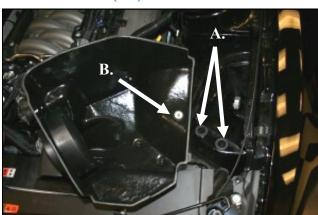
Locate and remove the Two Lower air box mounting grommets, and install them in the inner fender. B) Remove the Upper air box mounting grommet and steel off from the factory air box into the CAB. sleeve, and re-install into the Airaid CAB.
