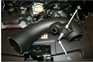
4. Install the Grommets and Fittings into the Airaid intake 5. Using the supplied Torx driver, remove the MAF sen- 6. Install the filter adapter (#6) using three 1/4-20 button transmission equipped vehicles will also use the 3/8" Fitting (#17) and 3/8" Grommet (#20). Manual transmission vehicles will not need the 3/8" components and will use the Blind Grommet (#21).
