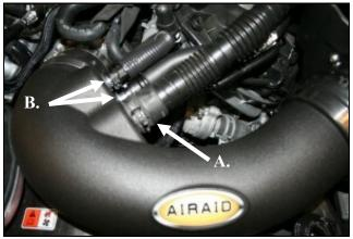
11. Install the Airaid Intake Tube into the couplers, and 12. A) Install the Airaid Premium Filter (#1) onto the tighten all Hose clamps. A) Reconnect the Resonator tube filter adapter and tighten the hose clamp. B) re install the to the Airaid Intake using the OEM clamp. B) Reconnect Resonator tubing into the factory Stand off. the breather line/lines to the Aluminum Fittings depending on your application. Apply the Airaid decal onto the Tube as shown.
